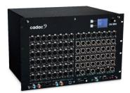
The Cadac CM-SR64 is 7U fixed configuration self-powered stage rack, featuring 56 Cadac mic-amps and 32 analogue outputs plus 8 AES3 inputs and 8 AES3 outputs. A 2.4" colour TFT displays the unit's menu structure along with an integrated headphone amp for local monitoring. The CM-SR64 connects to the console using Cadac's MegaCOMMS network protocol via coax cable or optical fibre.
