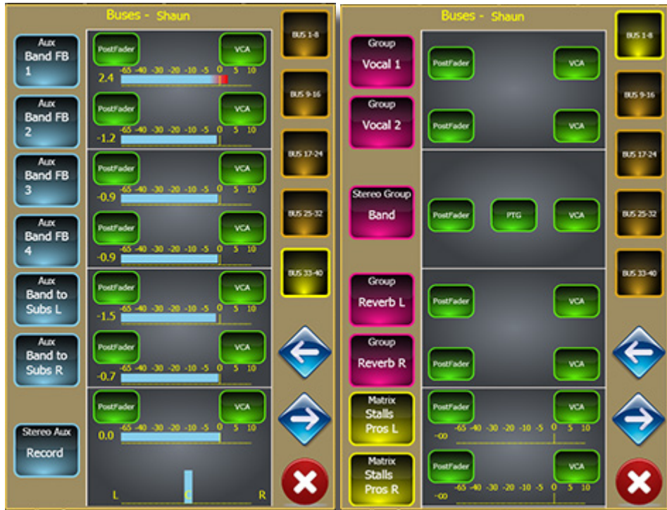
Examples of Aux, Group and Matrix busses.
