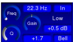
**Shelf** – switches the LF section of the equaliser between Bell and Shelving modes. In Shelving mode, the EQ section acts as a “bass” control, and has a fixed slope of 6 dB/octave. Default is **Bell**.
