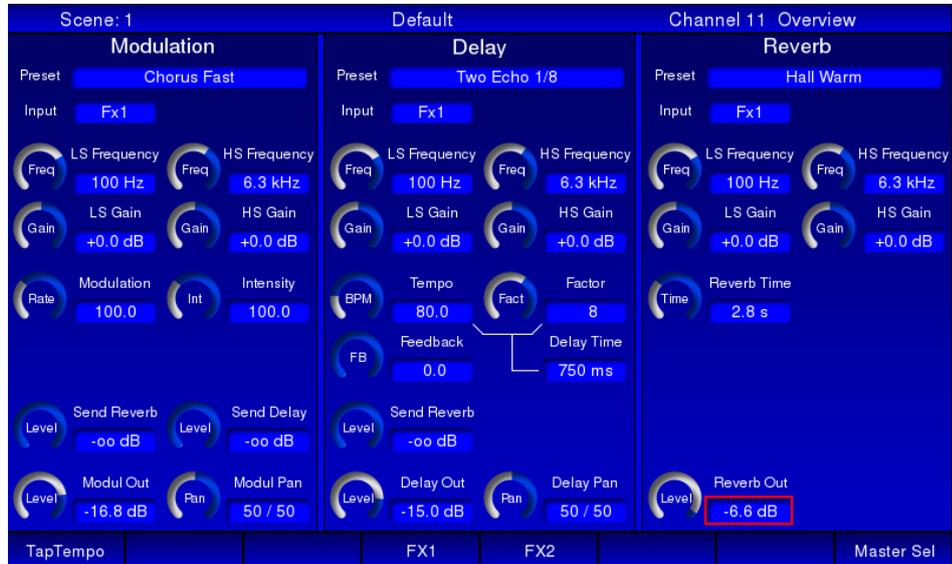
Each FX processor comprises three separate FX “modules”: Reverb, Delay and Modulation.
