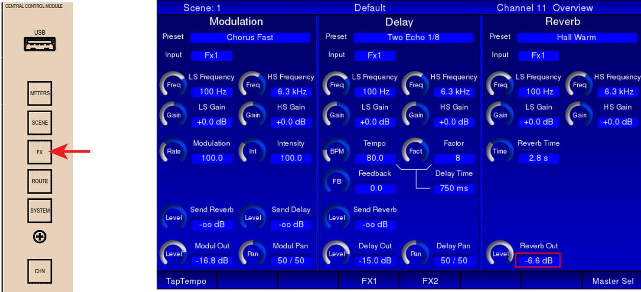
The processors’ inputs are two “virtual busses”, FX1 and FX2, which can be used in the same way as any of the Aux sends. The outputs may be routed to the stereo output and their FX return levels controlled by faders 13 and 14 when the OUTPUTS layer is active.
