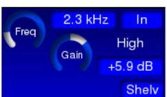
**Shelf** – switches the HF section of the equaliser between Bell and Shelving modes. In Shelving mode, the EQ section acts as a “treble” control, and has a fixed slope of 6 dB/octave. Default is **Bell**.
