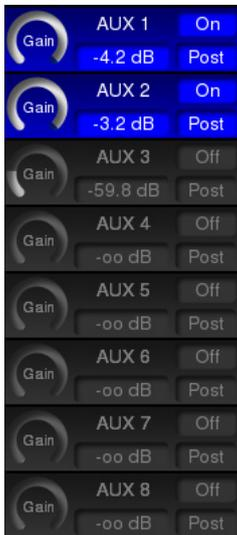
If a section of the channel processing is bypassed (e.g., gate, compressor, EQ, etc.), the screen display corresponding to the section is “dark” (greyed-out) to indicate it is not available. See left for example; only AUX 1 and AUX 2 are active.
