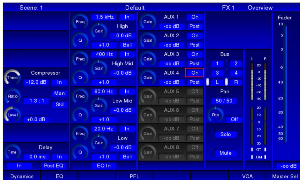
On the CDC FOUR, the FX channels have an almost identical set of controls to a mono channel, although they are treating a stereo signal; this includes EQ, routing and Aux sends. For this reason, only the differences from a mono channel are summarised below. The description of the mono mic/line channel applies in all other respects. Refer to Page 32 onwards for full details.
