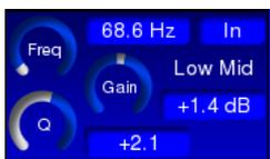
**IN** – switches the LF section of the equaliser into circuit. Default is **Out**.
