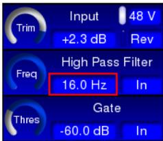
As channel parameters can be varied both from the TFT display or the CAM, a simple system of screen navigation is provided. On the CHN page, the virtual control corresponding to the last-adjusted control on the CAM is highlighted by a red rectangular cursor (see left).
