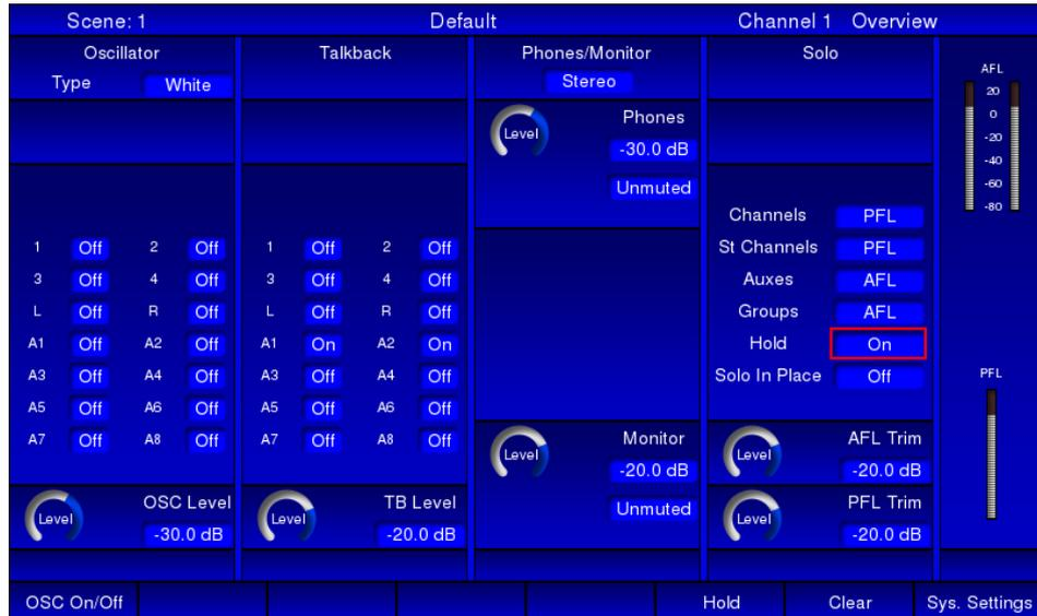
The System page provides controls for the CDC FOUR's oscillator, talkback routing, monitor control functions and Solo system control. The page is divided in four Modules, plus an area on the right for PFL and AFL metering. Most of the controls on these pages have no hardware equivalents, and are selected and adjusted by using the cursor keys and the **ADJUST** control.
