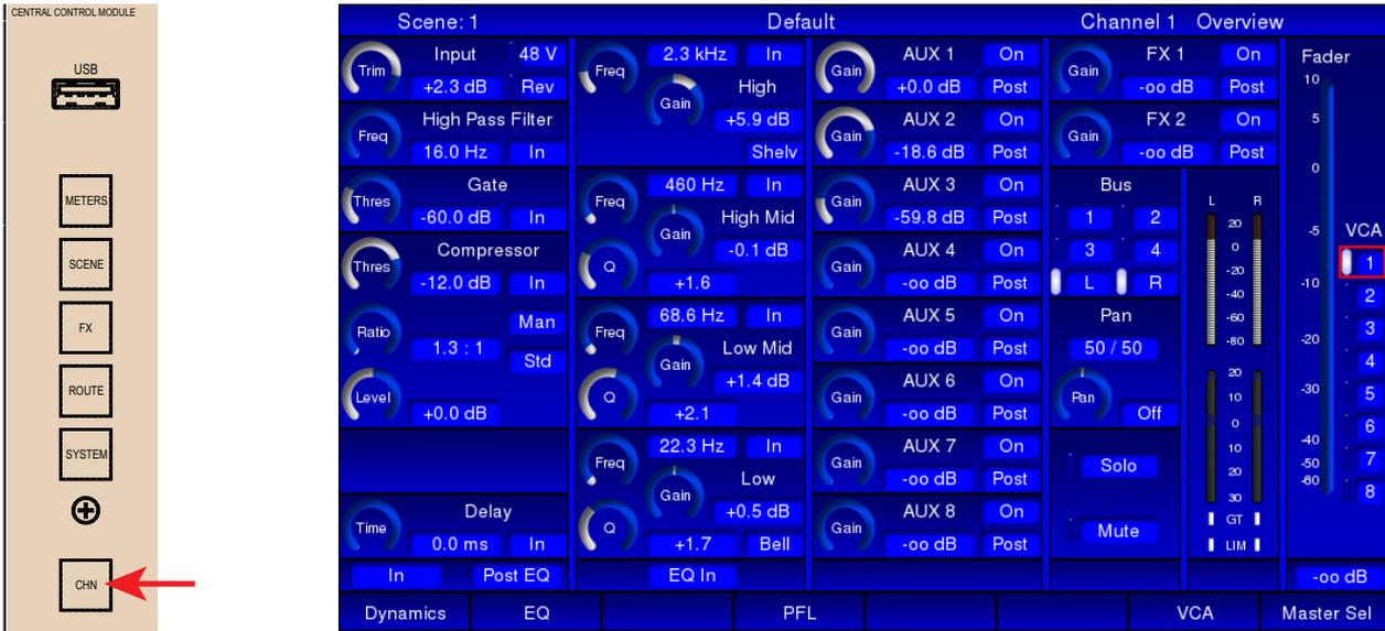
The screen shows a representation of a single channel strip. Every control on the CAM has a “virtual” equivalent on the display, and the page layout follows the conventional signal flow through a channel. It is divided into five vertical strips, the first four of which follow the layout of controls on the CAM. The fifth (rightmost) page strip shows the channel fader and VCA assignment.
