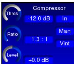
**VIN** – enables an alternative compressor algorithm which makes the compressor act like a leveller, modelling the sound of certain vintage compressors.
