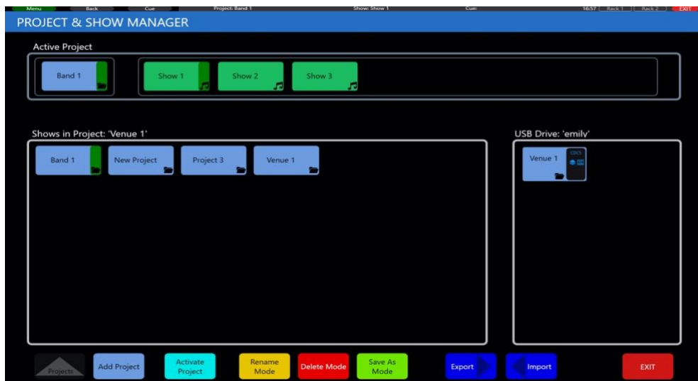
96: CM-Editor: Project and Show Manager menu allows the import and export of a Show to a USB key
