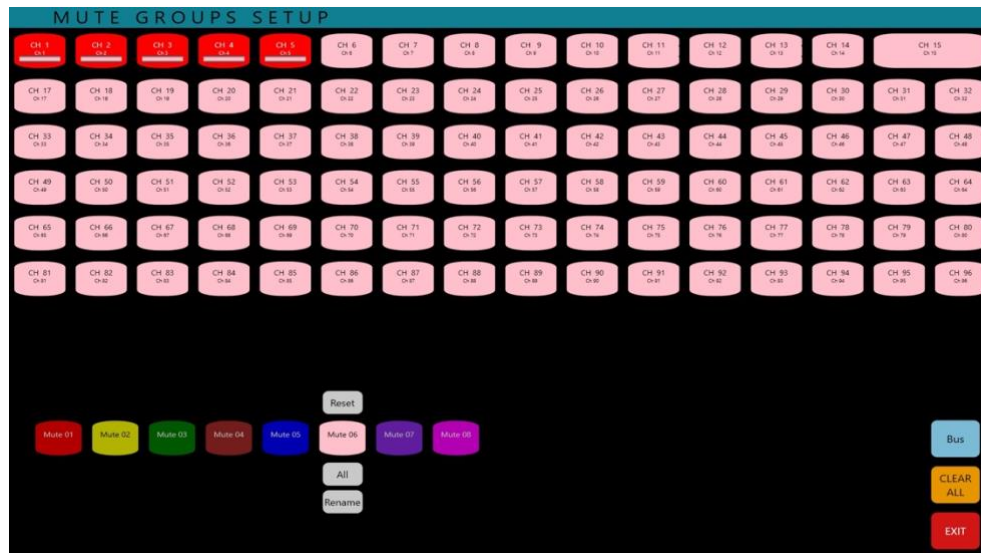
11: Mute Group setup screen. If a channel appears in more than one Mute group a colour bar representing the additional Mute Group appears under the channel number. Mute groups can also be re-named.
