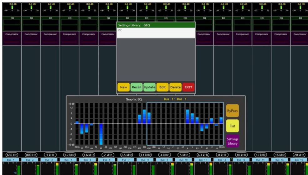
7: GEQ screen. The GEQ can be stored and recalled from the Settings Library
