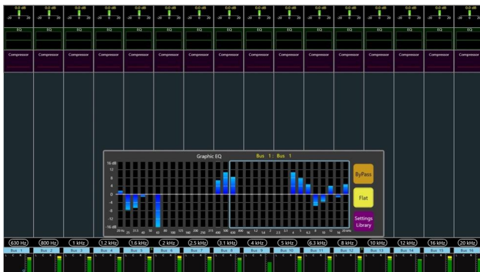
5: GEQ screen: The console faders control the levels of the EQ bands
