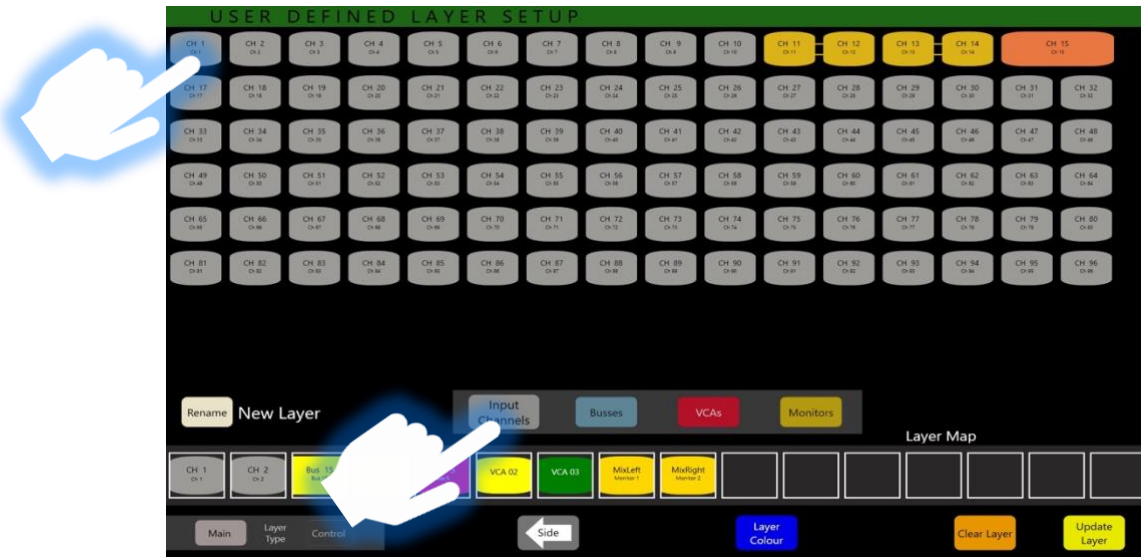
62: User Define Layer Setup: Select Input Channels, then select the input to be added to the customer layer
