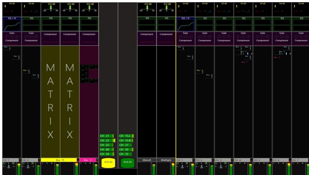
60: Custom Layers: 2 x input channels with 2 x VCAs, 2 x Busses, Mix left and right pinned to the screen
