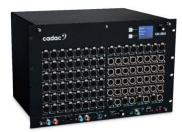
The Cadac CM-SR64 is 7U fixed configuration self-powered stage rack, featuring 56 Cadac mic-amps and 32 analogue outputs plus 8 AES3 inputs and 8 AES3 outputs. A 2.4" colour TFT displays the unit's menu structure along with an integrated headphone amp for local monitoring. The CM-SR64 connects to the console using Cadac's MegaCOMMS network protocol via coax cable or optical fibre.
