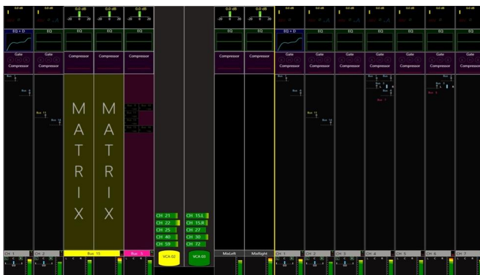
56: Custom Layers: 2 x input channels with 2 x VCAs, 2 x Busses, Mix left and right pinned to the screen
