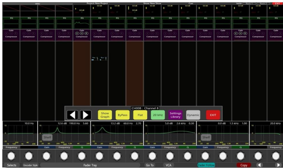
111: CM-Editor: The PC displays the same GUI as the console, but with virtual encoders. Quick access buttons to the Go To, VCA, Fader Follow, Selects, Copy functions plus virtual Faders are available at the bottom of the screen.
