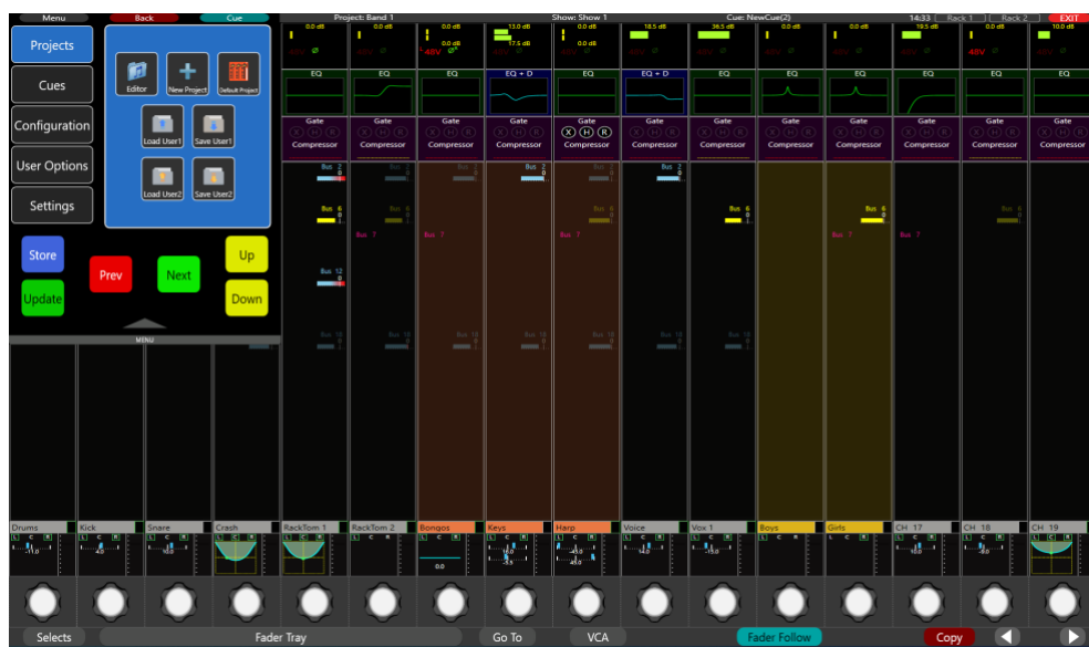
113: CM-Editor: The Control Screen window is accessed by selecting the Menu button at the top left of the displayed. This gives access to the menu structure that is found on the console's 6.5" physical displayed, along with the Back and Cue buttons.
