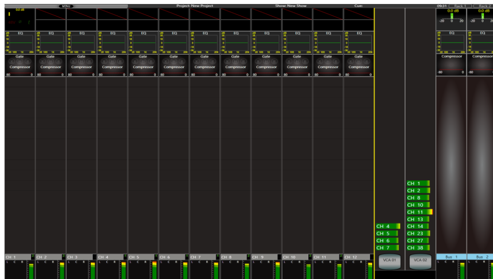
39: CUSTOM LAYERS: Inputs with 2 x VCAs and 2 x Busses pinned to the screen
