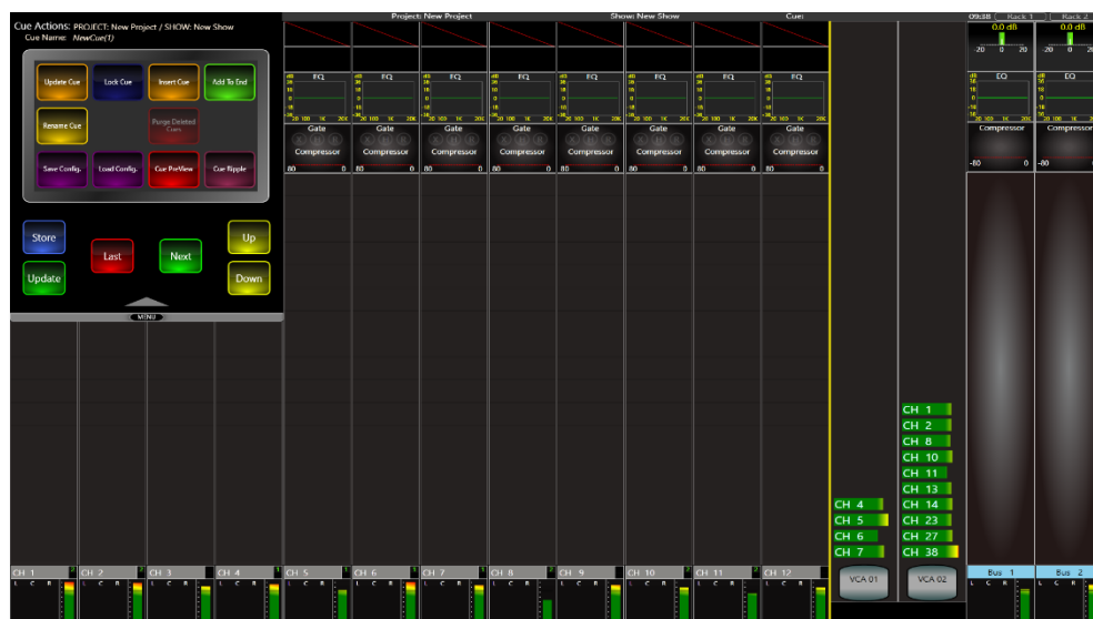
45: MENU SCREEN displaying the CUE options displayed by double taping a CUE or pressing the STORE button
