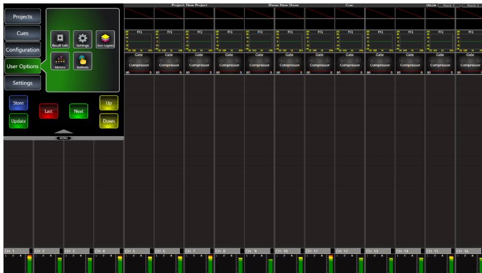
31: Virtual Meters show at the bottom of the Channel Strip. Meter Options can be found in the USER OPTIONS in the MENU Screen.
