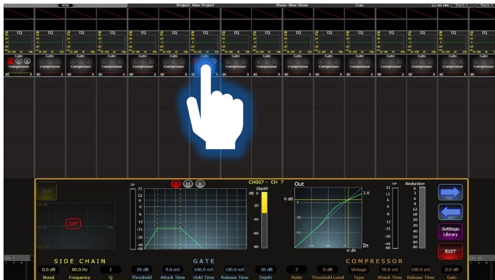
25: DYNAMIC interface populates the screen when the DYNAMICS on the "channel" strip is pressed
