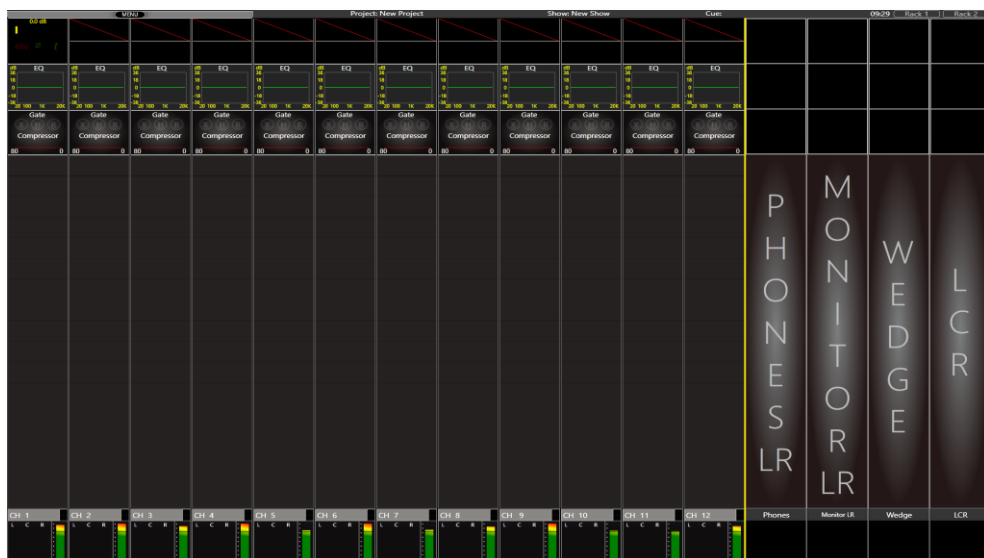
5: DEFAULT MASTERS - a default USER ASSIGN button. Four faders now act as PHONE LR, MONITORS LR, WEDGES and LCR
