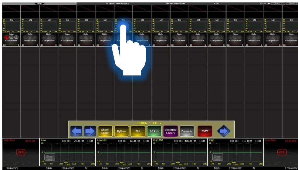
24: EQ controls populate the screen when the EQ on the "channel" strip is pressed
