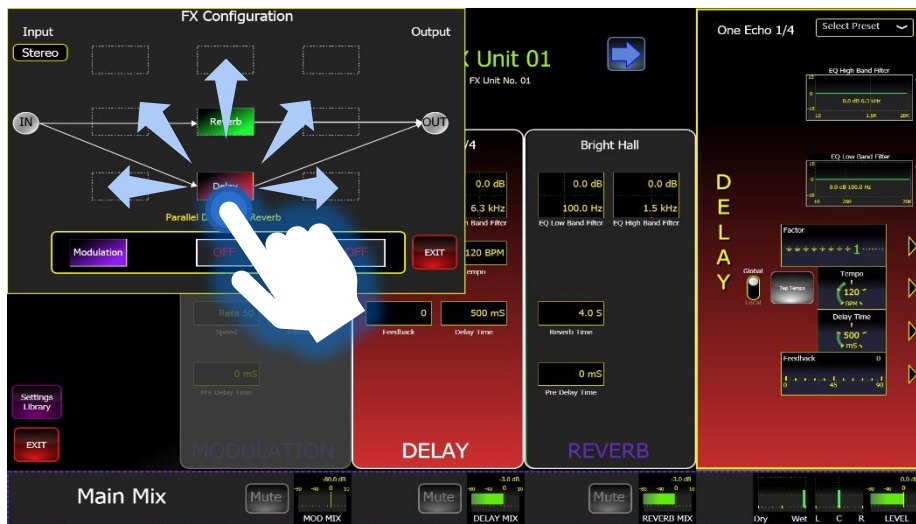
42: FX build screen - select the element (a choice of reverb, delay and modulation) and drag and drop into it one of the possible 9 "slots"
