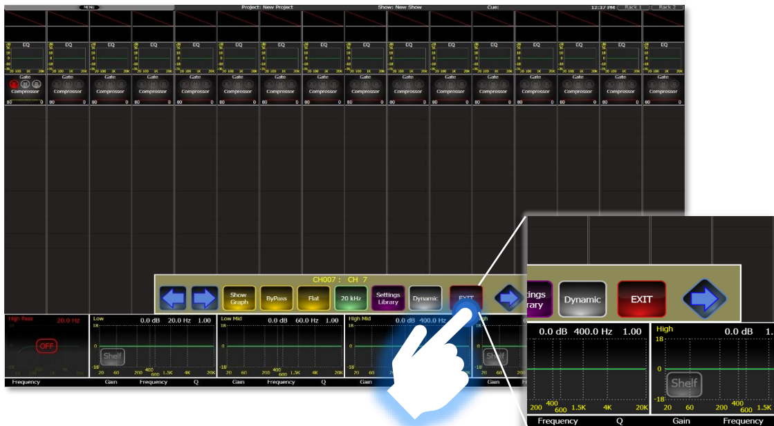
26: EXIT closes the function, or window, and removes any mapping to the encoders
